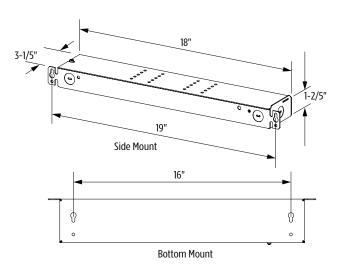
Remote driver boxes have knockouts for conduit connections
