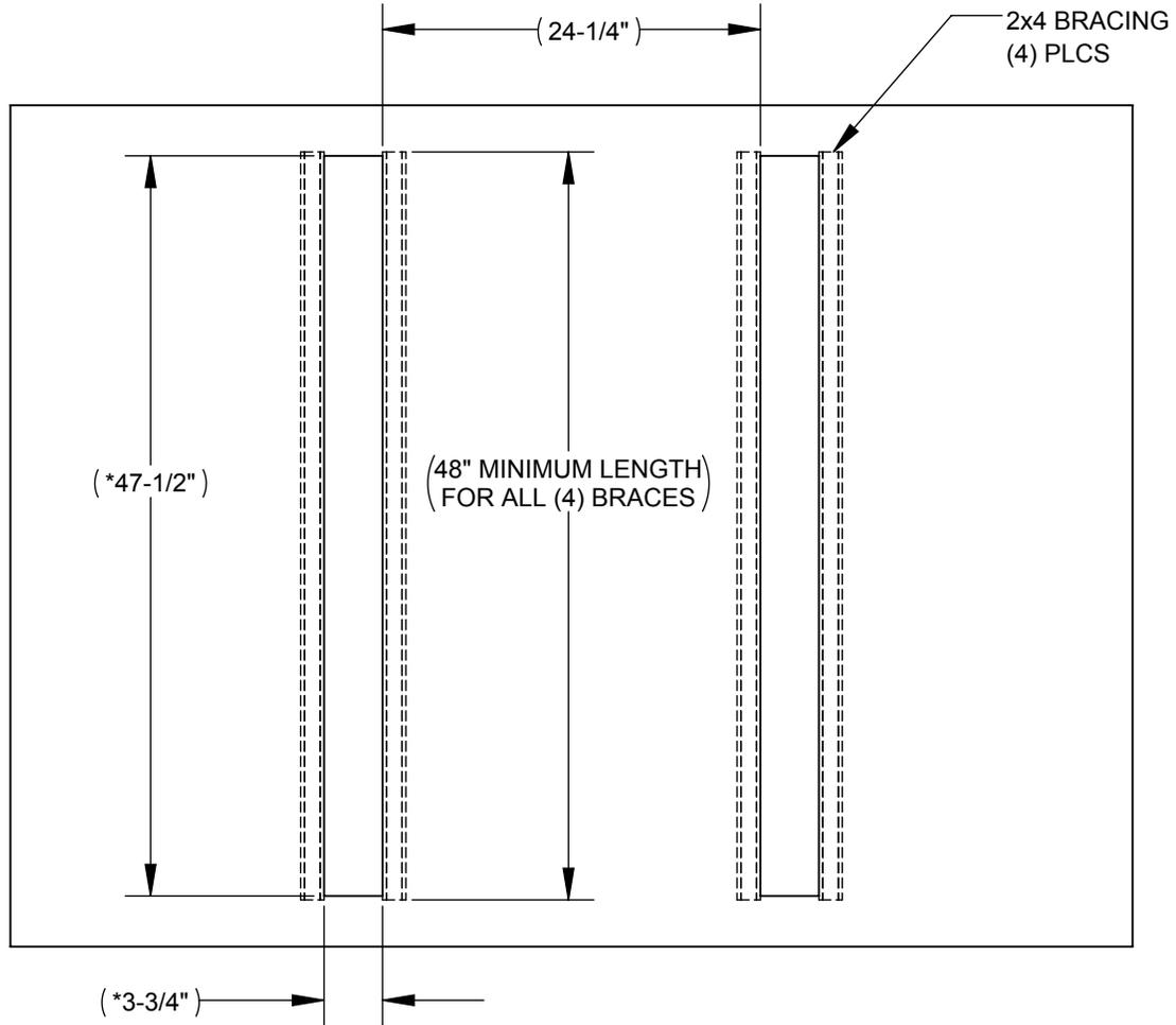
CUTOUT FOR FIXTURE MUST BE EXACT TO THE DIMENSIONS SHOWN
