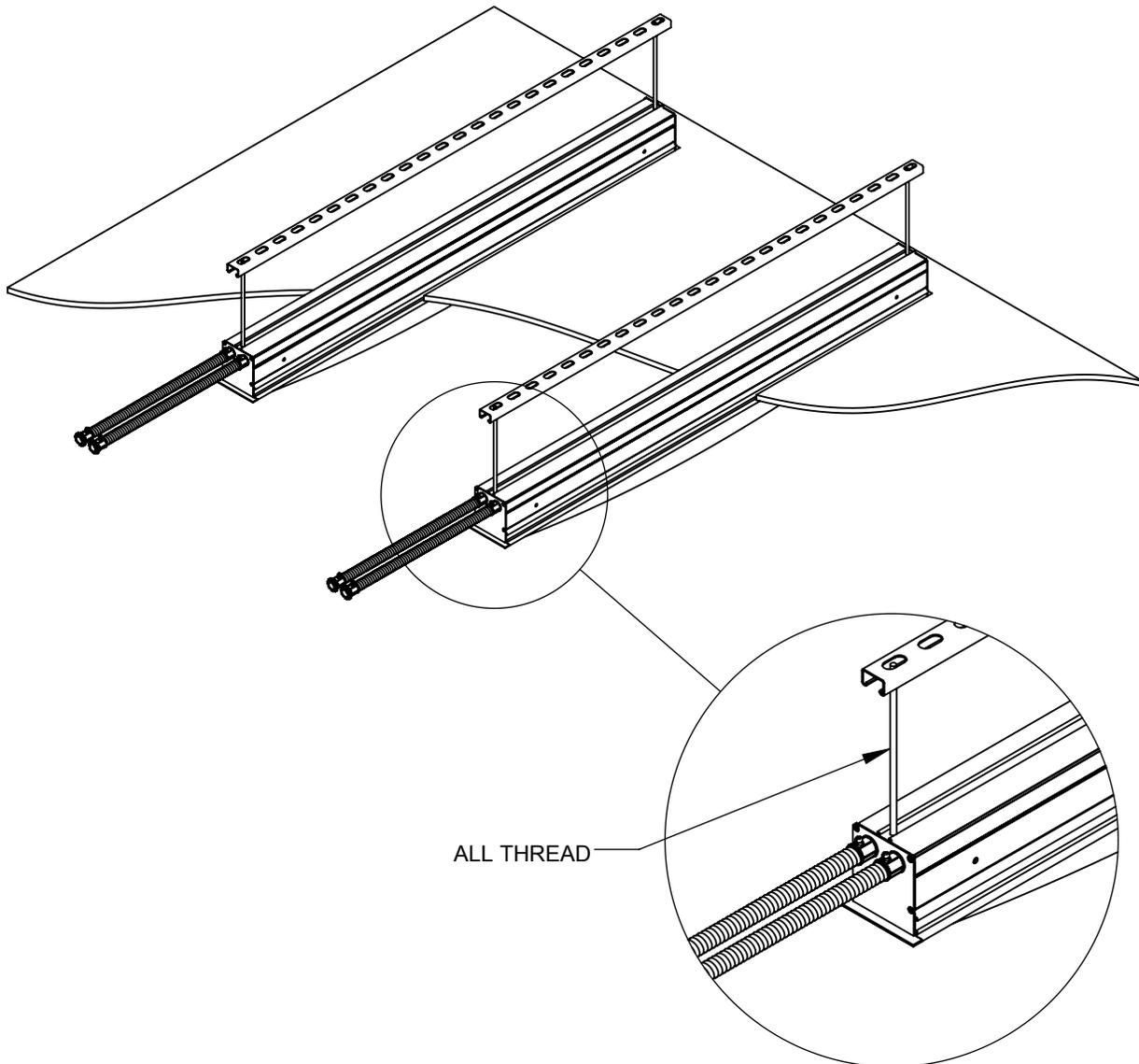
1. If connection to building structure is required, use holes on top of fixture.
