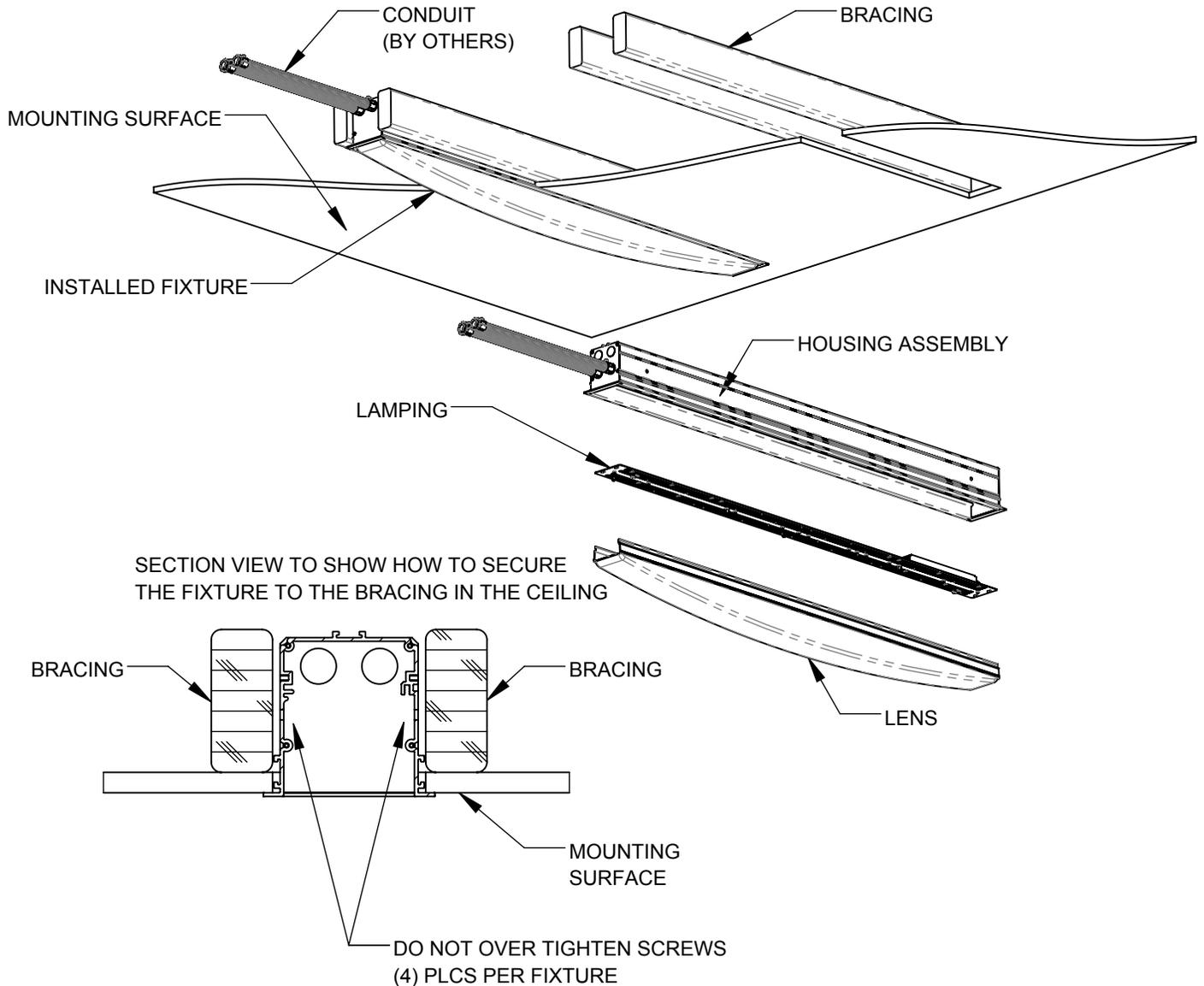
1. After cutting the proper size holes (see page 5) in the drywall, install the bracing.
